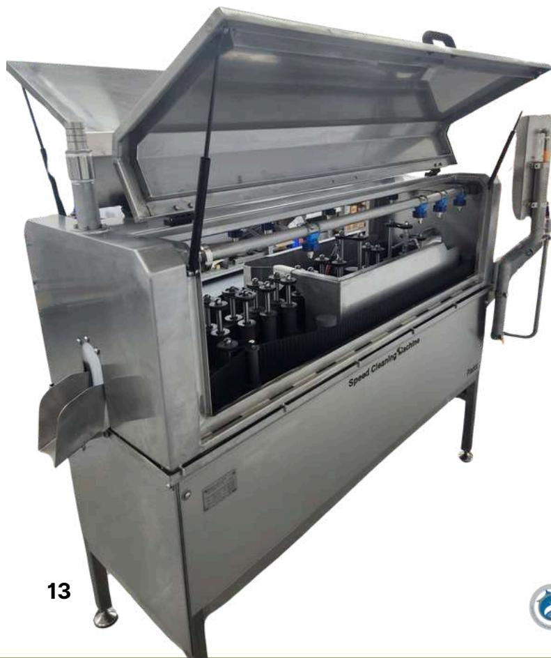
The Speed Cleaning Machine revolutionizes the fish farming industry with its innovative use of high-pressure water jets to clean up to 28 fish per minute efficiently and precisely.
